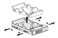
4 Align the new hard disk with the HDD carrier, then secure it with the four screws you removed in step 3-1.
